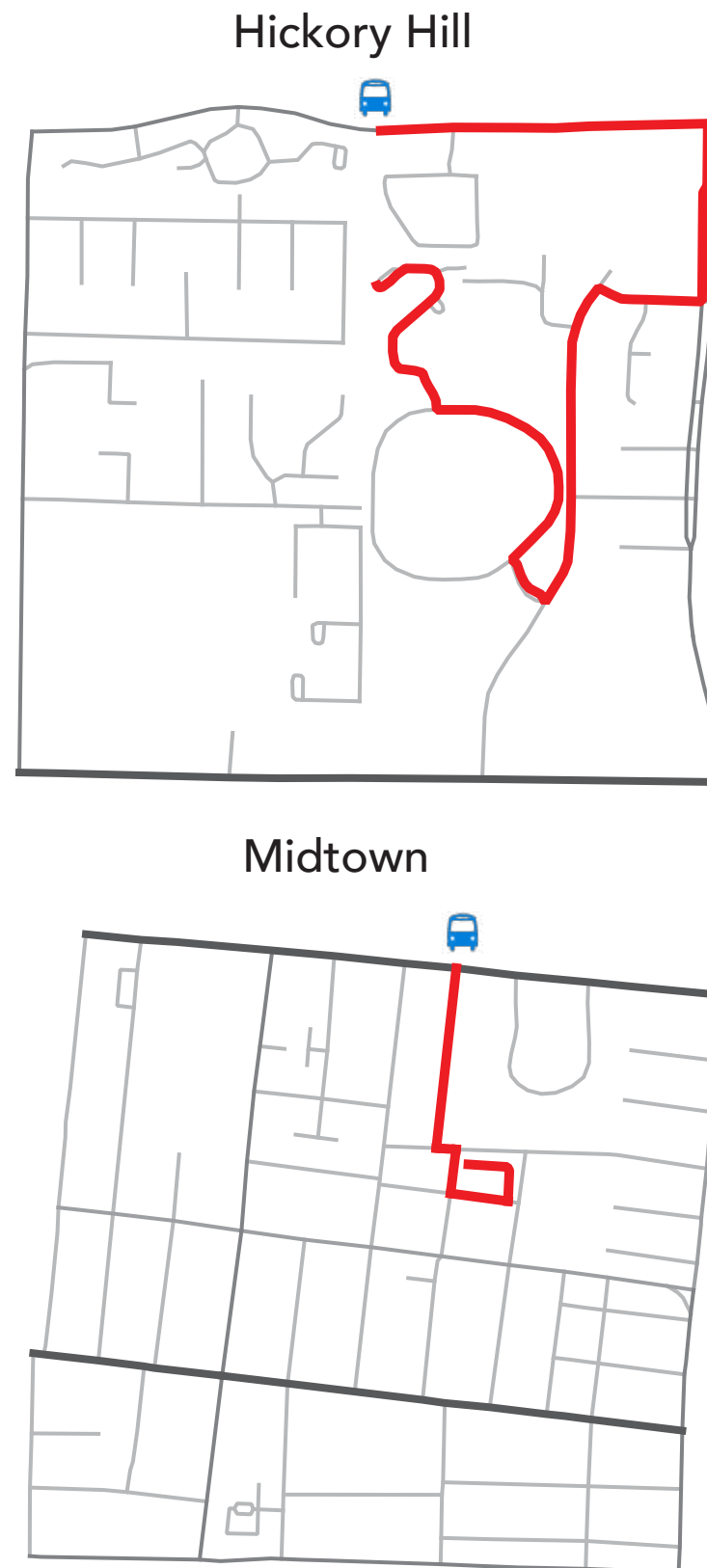
Figure 17: Differences in walkability in two Memphis neighborhoods. Red lines show the longest-case walking paths for access to a bus stop that would be a short “flying distance” away.
